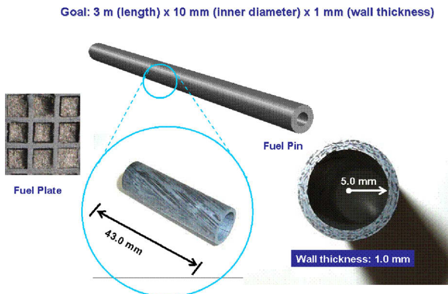
Fig. 4. SiC/SiC fuel pin or fuel plate for GFR.
